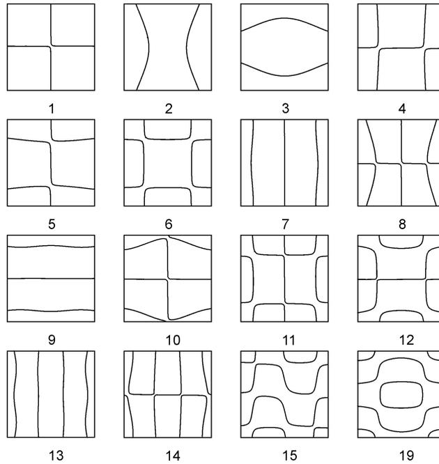
**Figure 3.** Vibration modes  $(m, n)$  of cross-ply laminated plate PU10.
