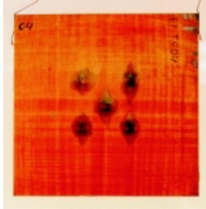
Figure 16. Damaged cross-ply laminated glass/epoxy plate after 5 impacts.
