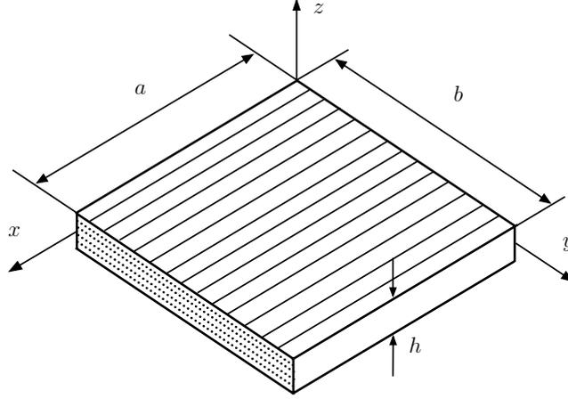
**Figure 4.** Unidirectionally reinforced carbon/epoxy plate.
