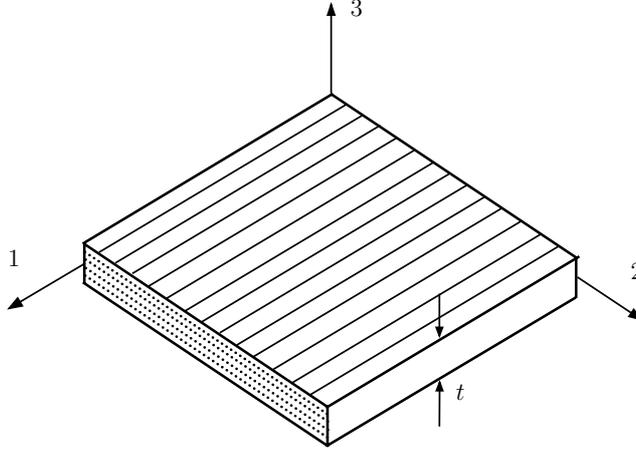
**Figure 2.** Single layer of laminated plate.
