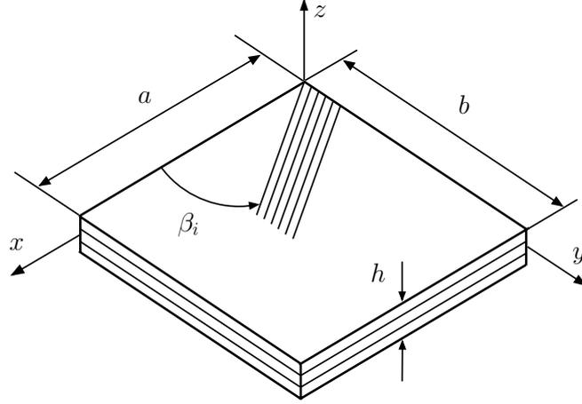
**Figure 1.** Geometry of laminated plate.
